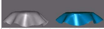
3-D digital images of a sample fabric (blue), and simulated drapes (grey).
