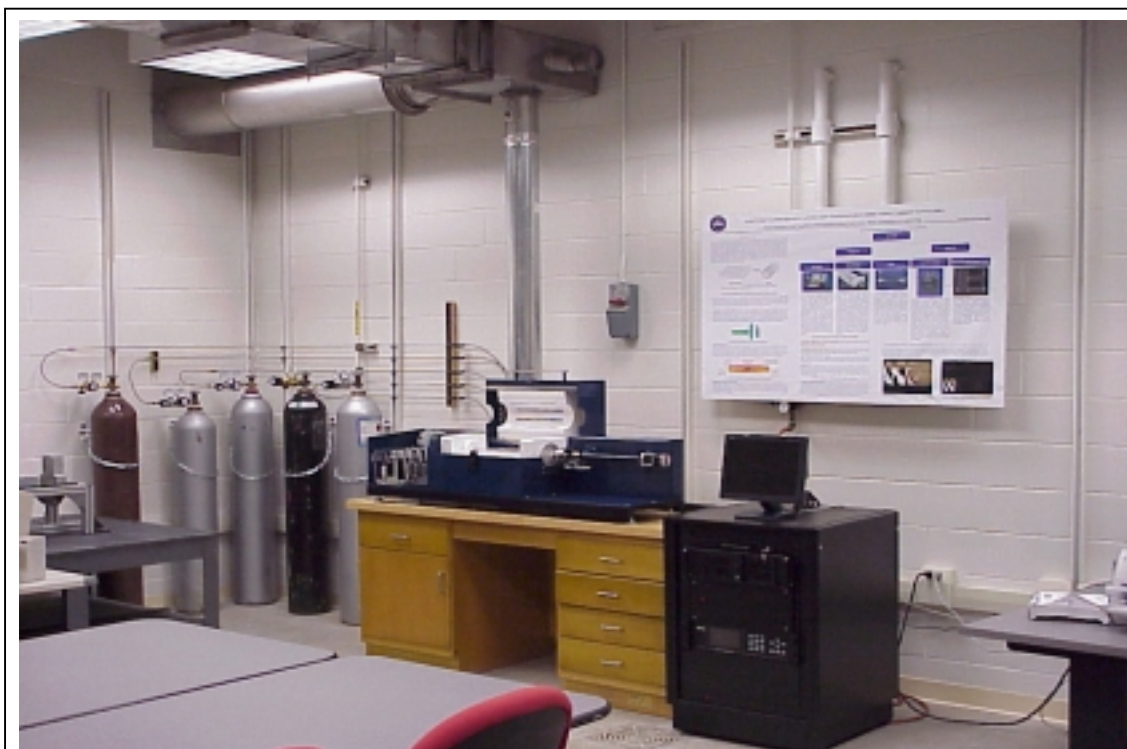
Fig. 4 Easytube™ CNT synthesis and fabrication station housed in Smart Structures and NEMS Lab (acquired by both PIs and Clemson Univ. resources for feasibility study during the course of M03-CL07s).
