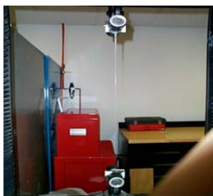
Figure 1. A superb drawability (4000 %) of N66-GaCl 3 film on Instron. The initial film length was 3 cm.
