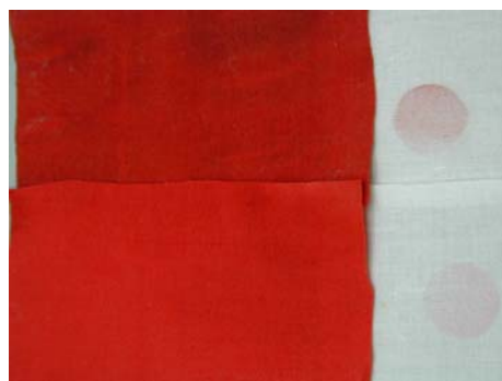
Figure 1. Image of 'azoic' dyeings on cotton using pressurized CO 2 (top: 3000 psi, 80 °C; bottom: 860 psi, 25 °C).
